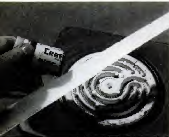
In an emergency you can improvise a good electrical insulating tape by coating a cloth strip with cement
